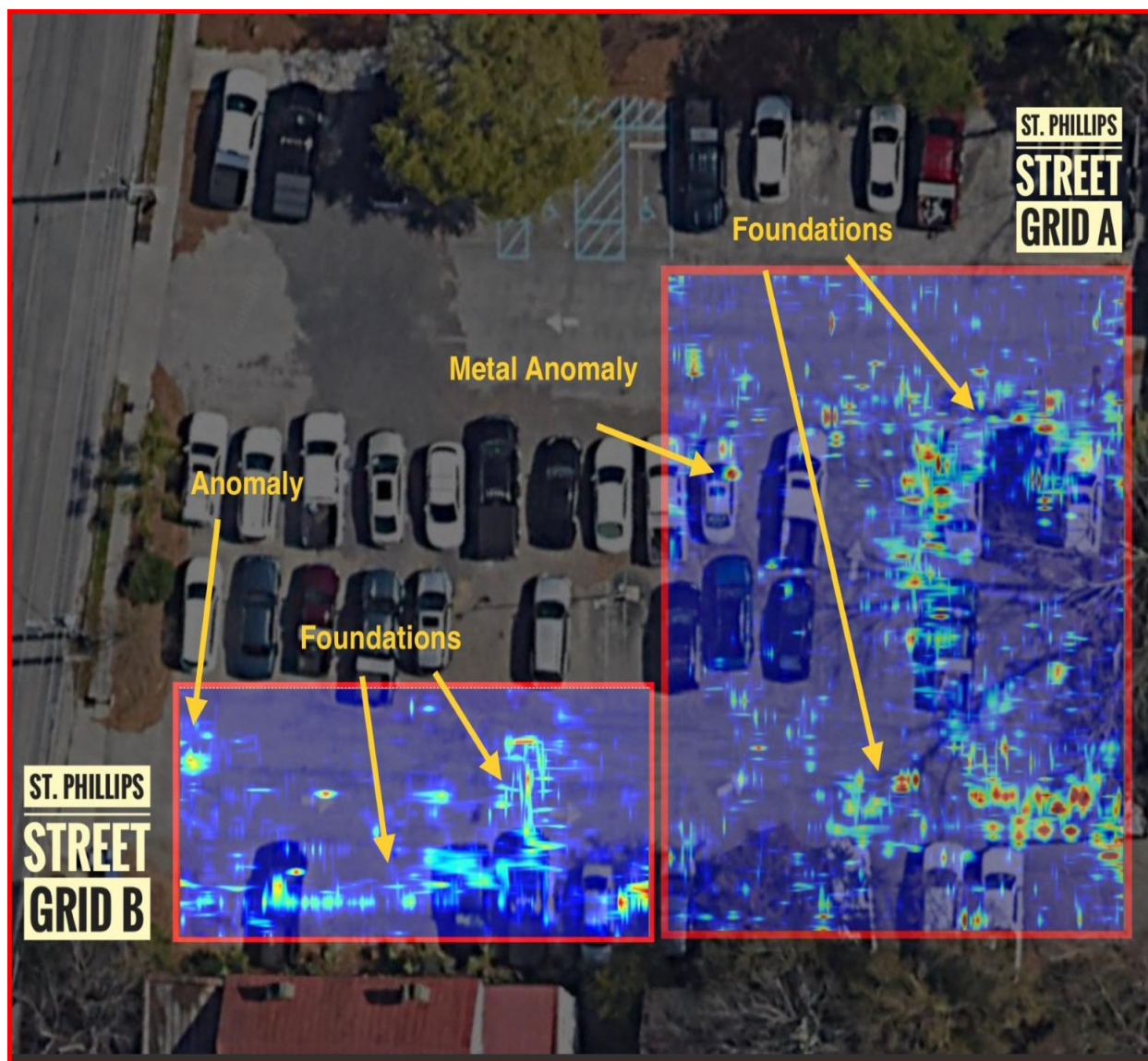
Figure 20. GPR results at 99 St Philip Street.
