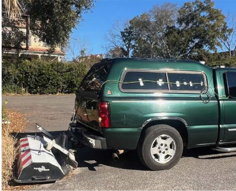
Figure 8. The Talon GPR is mounted to the rear of the vehicle. The GPS is centered over the cab. (photo by M. Scott Harris)
