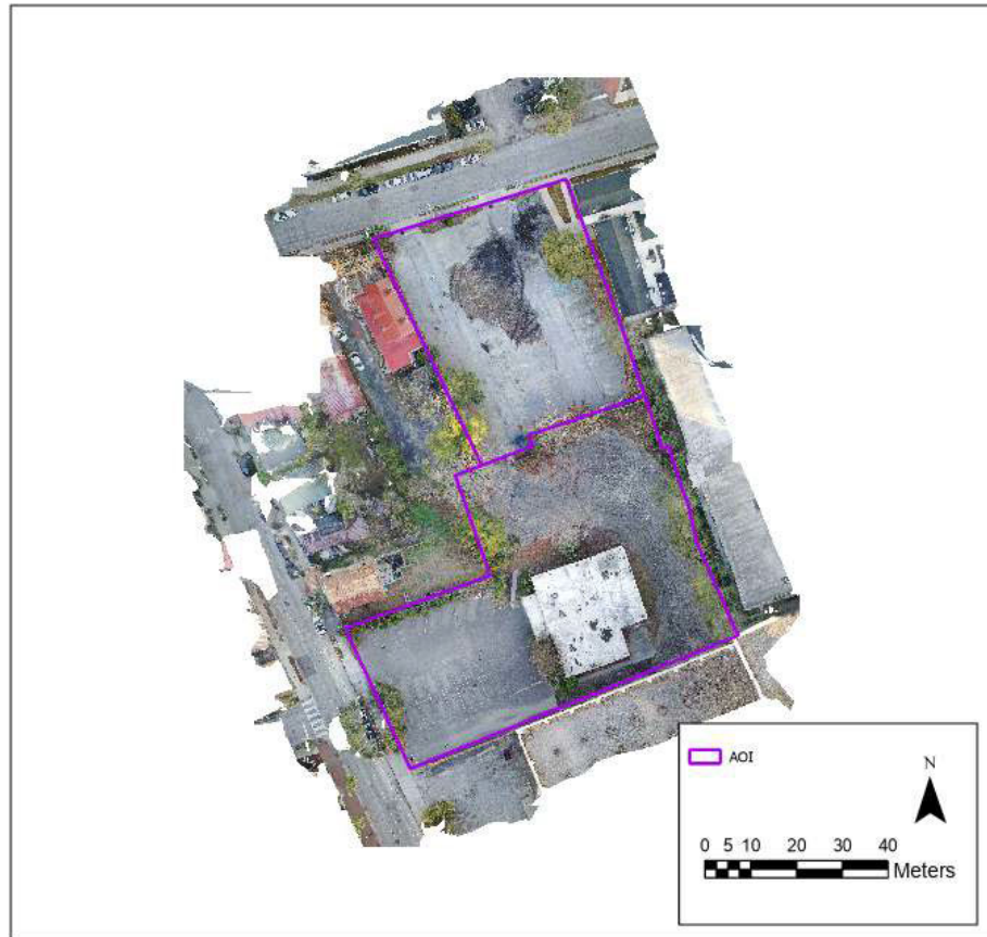
Figure 15. Georeferenced orthophoto mosaic of the AOI. Image has 1-cm pixel size.
